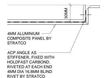
SECTION A - STIFFENER EDGE FIXING
